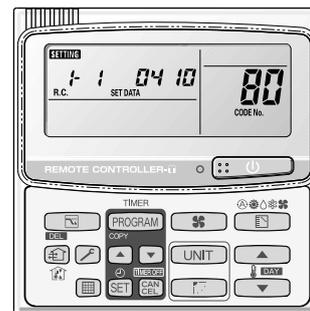
**80** : <Refrigerant type> ㉑ and ㉒ are displayed alternately. (Example shows 0000 0410 (R410A).)
