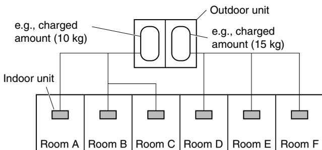
The possible amount of leaked refrigerant gas in rooms A, B and C is 10 kg.
