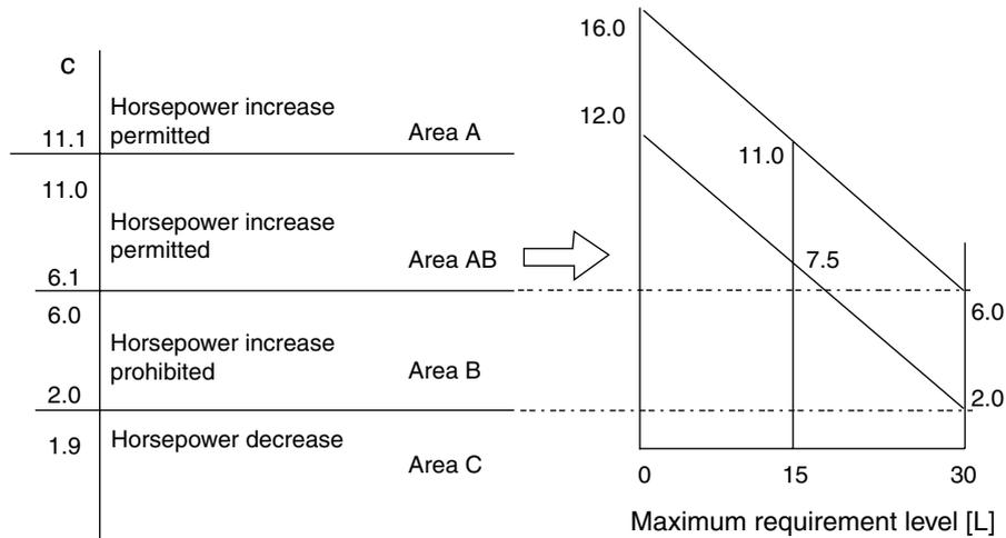
\* Depending on the maximum requirement level of the indoor unit, the judgment temperatures for each area may vary as shown in the figure (example).
