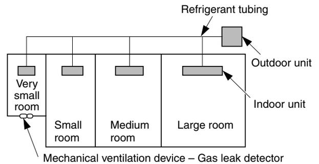
3. The minimum indoor floor space compared with the amount of refrigerant is roughly as follows: (When the ceiling is 2.7 m high)
